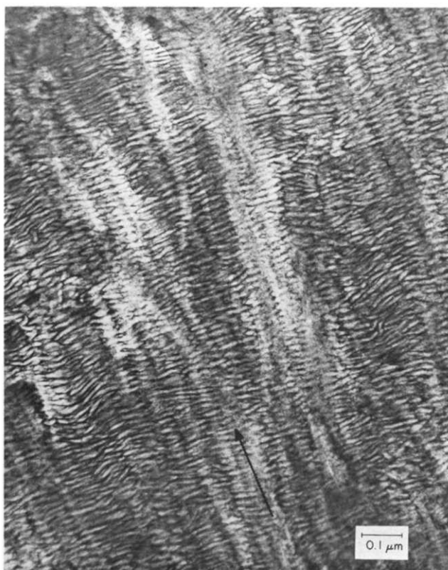
Figure 6 Electron micrograph of a thin section cut parallel to the extrusion direction (arrowed). The structure is stained by uranyl acetate. The fine striated structure corresponds to lamellae seen edge on, where the stained amorphous regions appear dark
