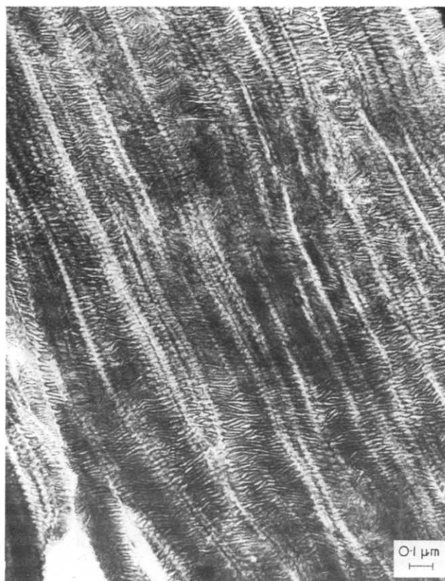
Figure 7 Electron micrograph of a more heavily stained sample revealing the overall columnar structure with central backbones
