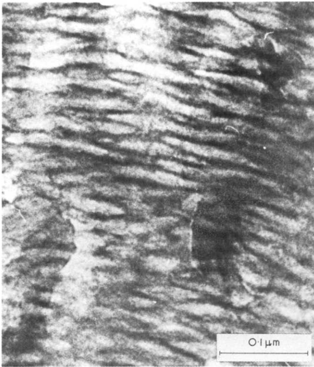
Figure 14 A high magnification electron micrograph of a lightly stained section, showing interlocking tapering lamellae
